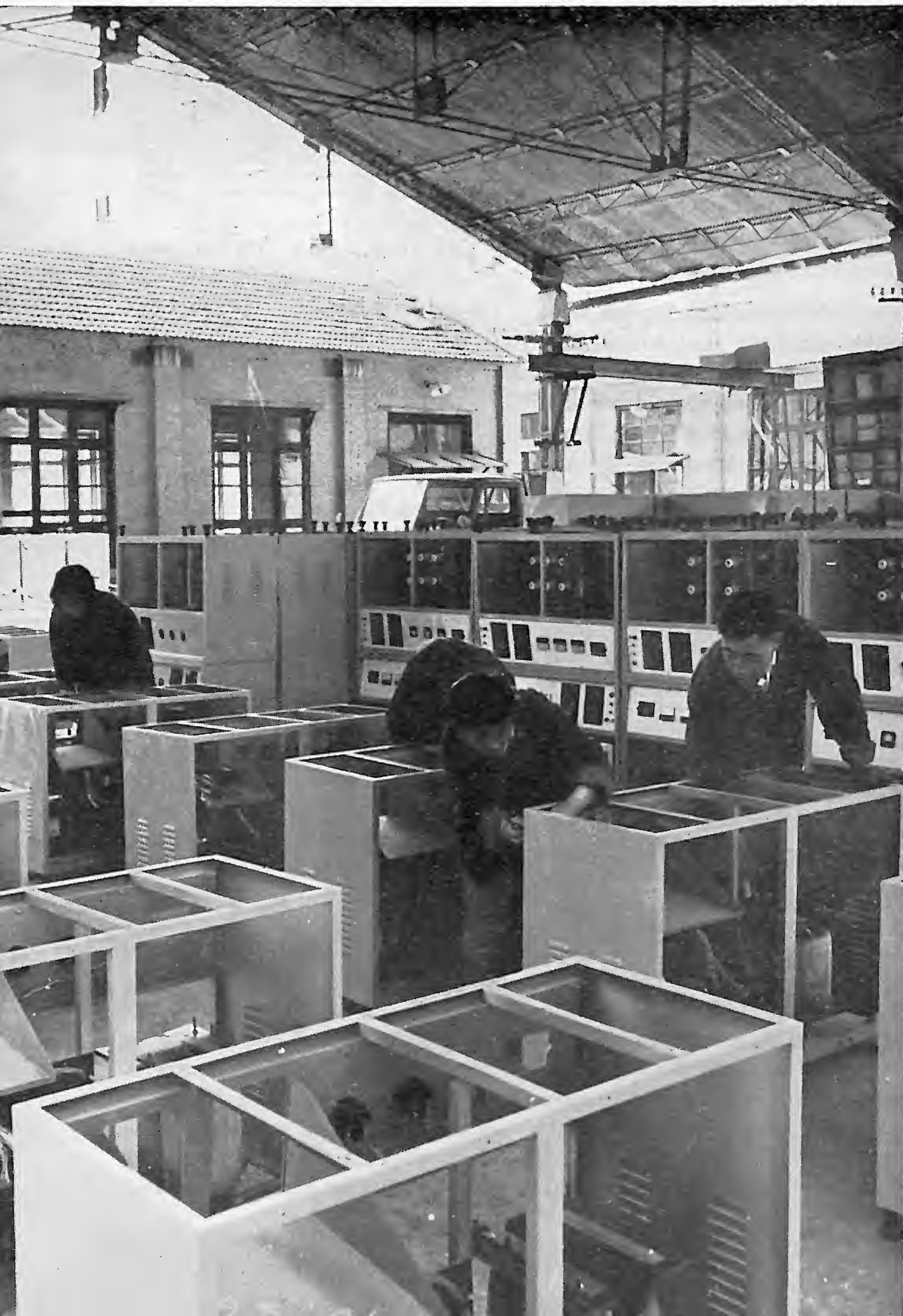
Assembling diffusion furnaces.
